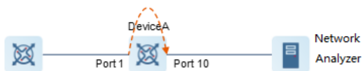
Figure 2-7 Operating Principle of Port Mirroring
